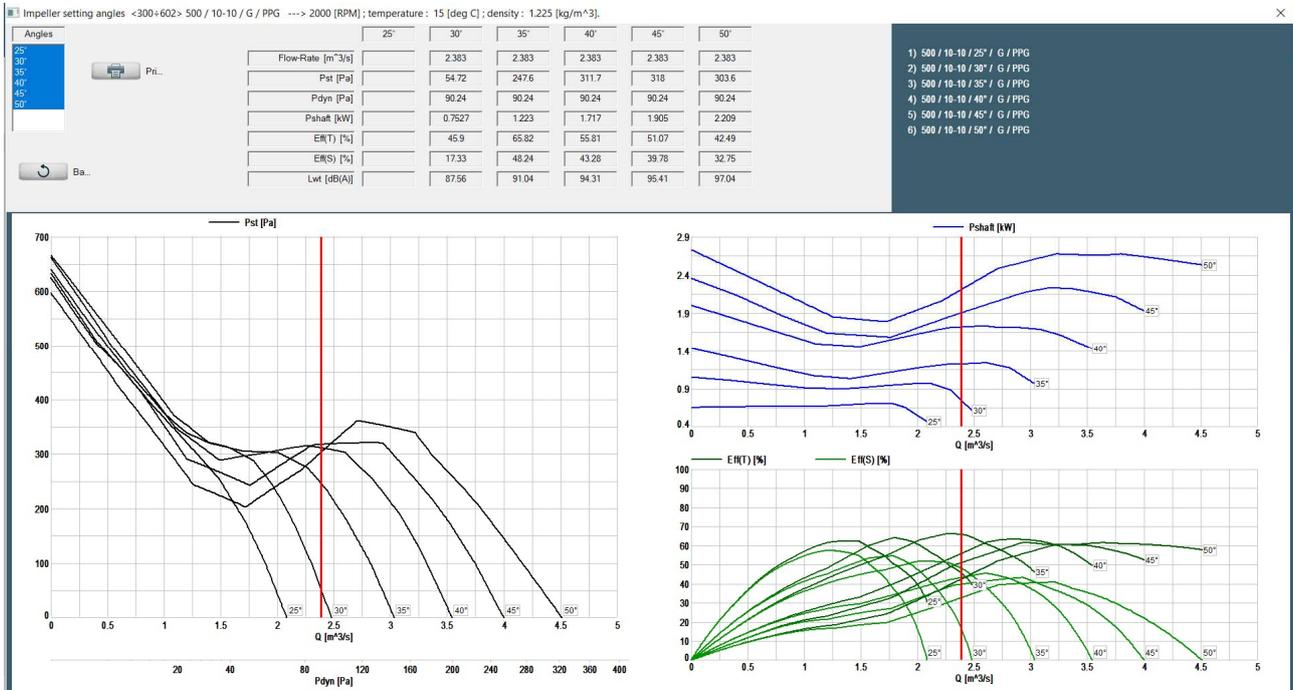
Figure 29 Performance of an impeller at different setting angles
