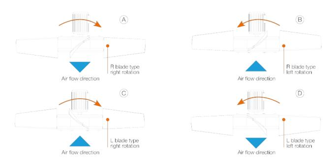
HasconWing blades are manufactured with leading right edges (R) and leading left edges (L).
