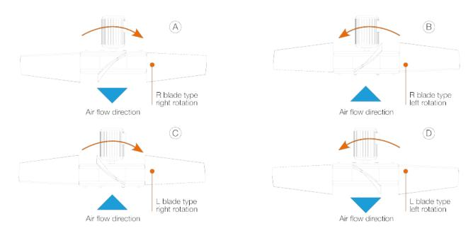
HasconWing blades are manufactured with leading right edges (R) and leading left edges (L).
